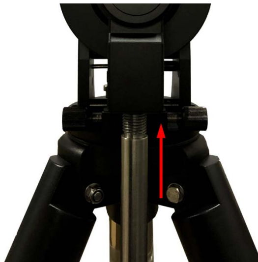
Figure 18. Install CW shaft
