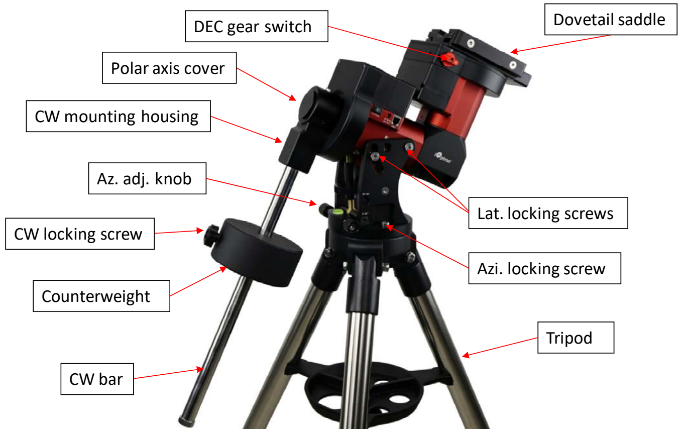
Figure 1.CEM40 mount assembly
